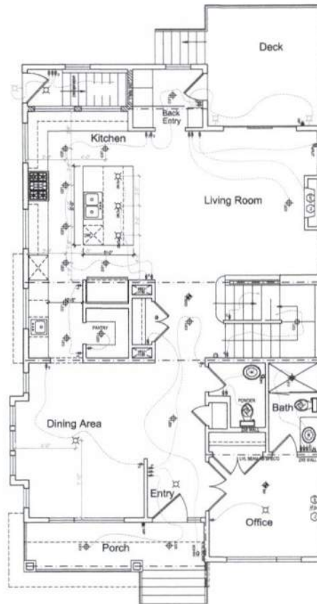
main floor electrical plan
